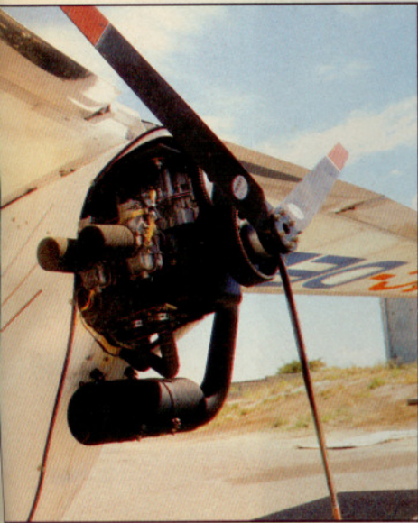
Dual carburetors are optional on the Rotax 503 (above). Engine provides cabin heat and 12-volt electrical power.
